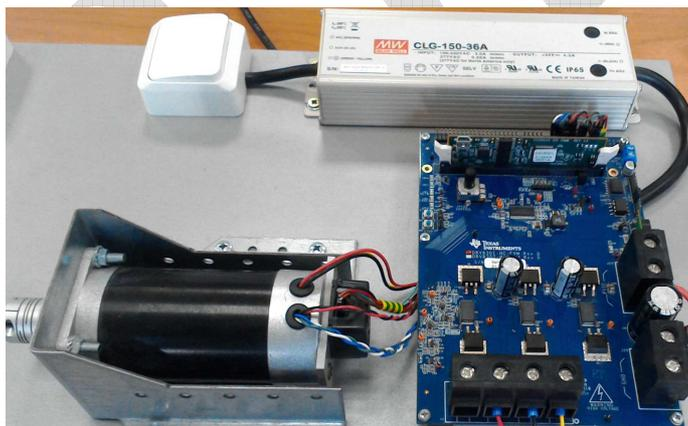
Figure 8. Motor kit with the PMSM and 1000 ppr incremental encoder.
