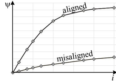
Fig. 3. Magnetisation curves for aligned and misaligned positions.
