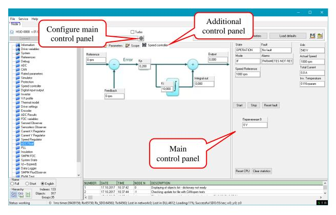
These panels can be managed through the device profiles setup window (see section 7.4.2 "Profile main options setting" above):
