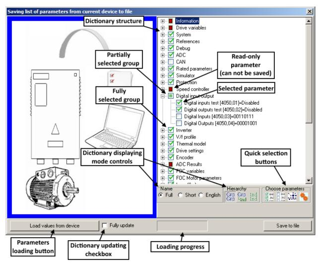
Fig. 6.7 Parameters saving window
